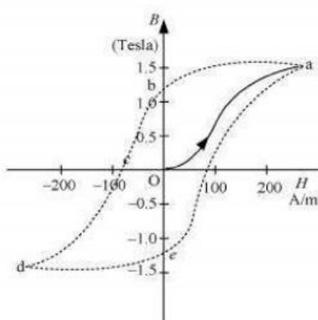
**(a)** It can be observed from the given curve that magnetisation persists even when the external field is removed. This reflects the irreversibility of a ferromagnet.
